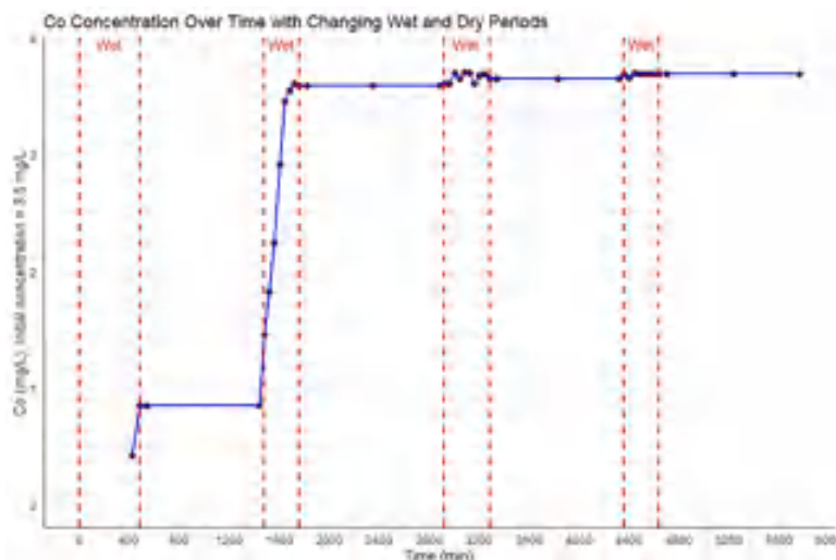
Figure 4-33 Breakthrough curve of Co 2+ concentration performance in the sand column of the SAT system during wet and dry periods
