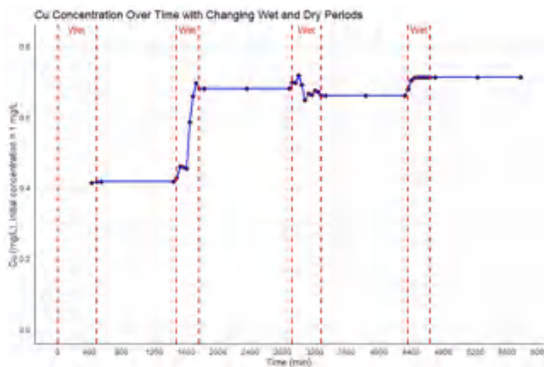
Figure 4-21 Breakthrough curve of \text{Cu}^{2+} concentration performance in the sand column of the SAT system during wet and dry periods
