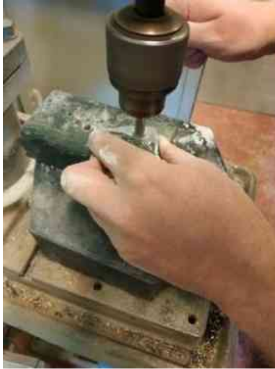
Figure 16 Taking small plug from the sample by using cylinder column drilling machine (edited by H.A.).
