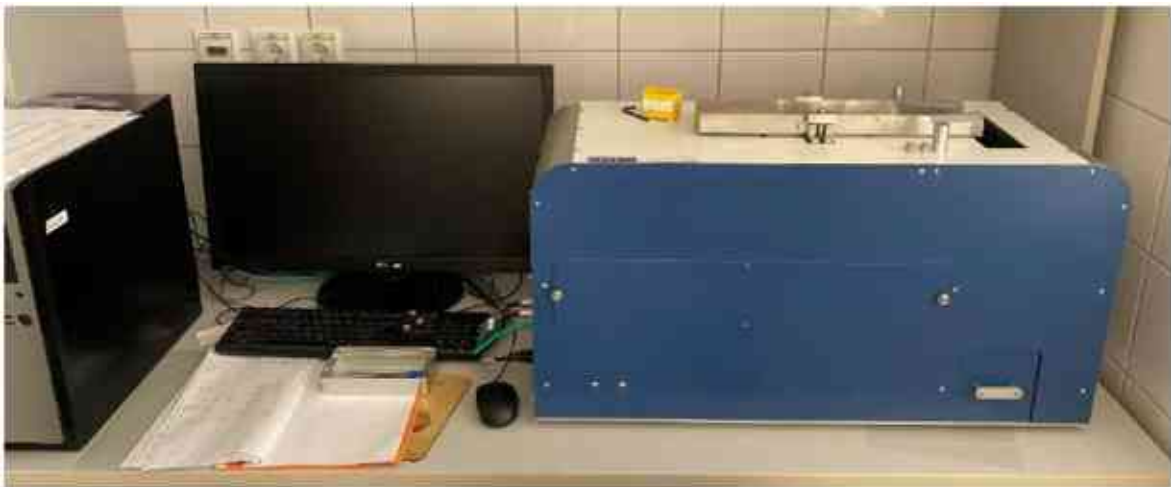
Figure 13-24: Occhio Zephyr ESR 2 equipment used during proppant size distribution, sphericity and roundness measurements
