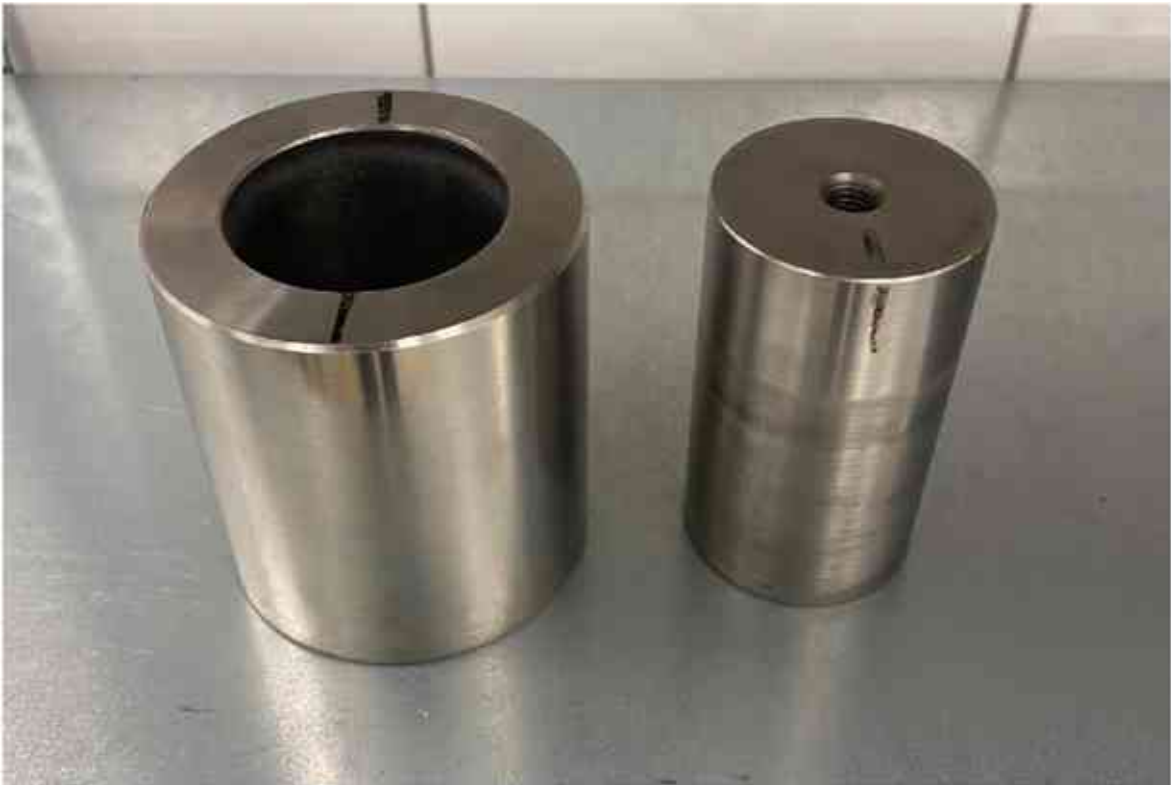
Figure 13-48: API RP 19C crush test apparatus used for bulk density measurements
