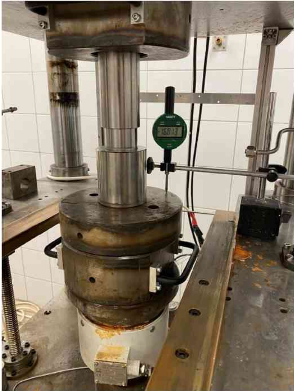
Figure 13-49: Bulk density measurement setup
