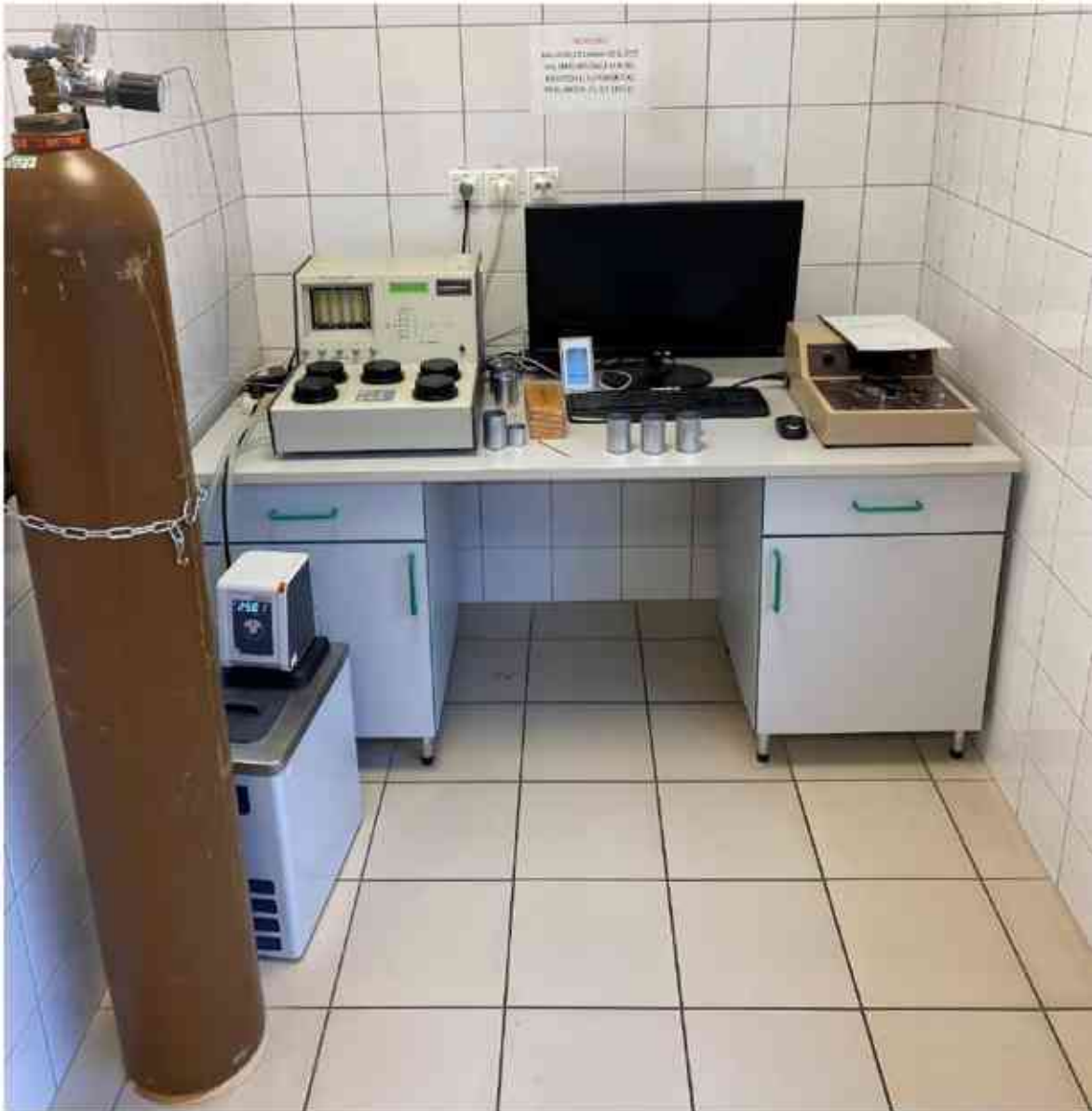
Figure 13-22: Pentapyc 5200e device used for specific gravity measurements
