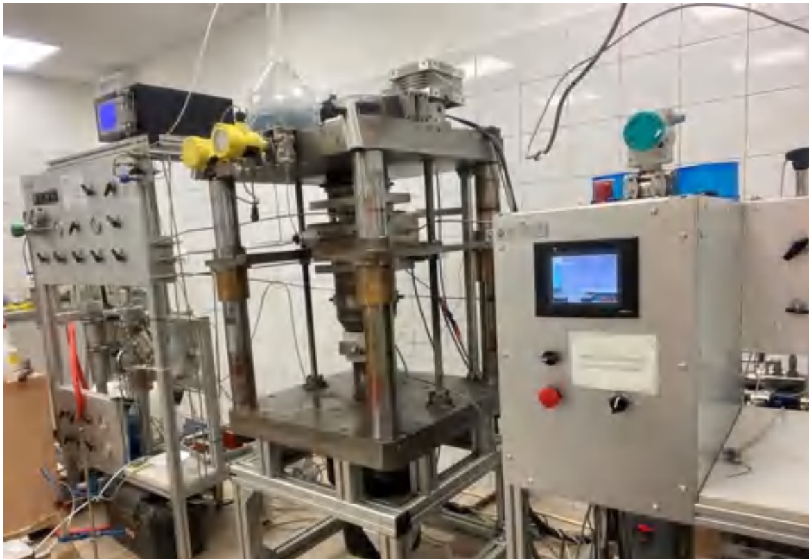
Fig. 74 Fracture conductivity measurement system in GEOCHEM's laboratory (edited by the Author)
