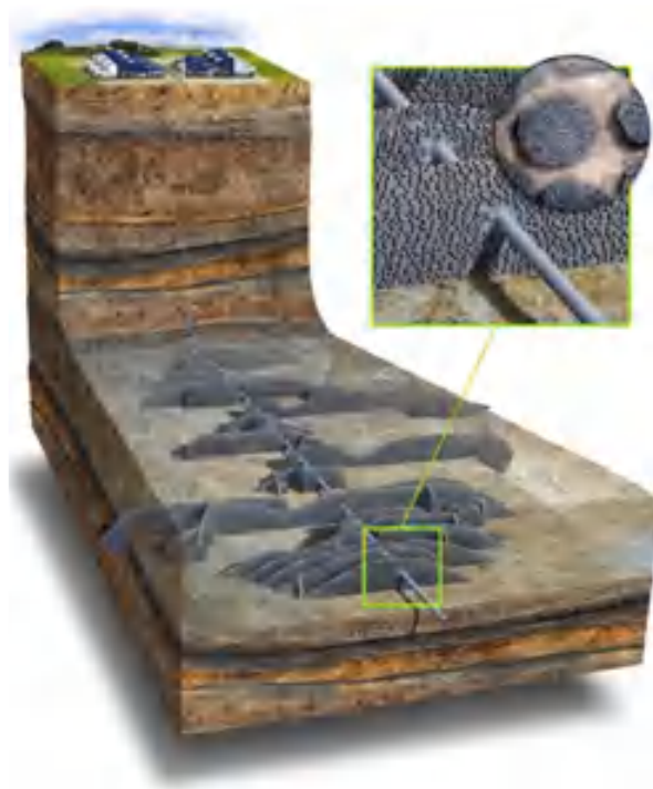
Fig. 1 Schematic of hydraulic fracturing (Schlumberger, 2021)
