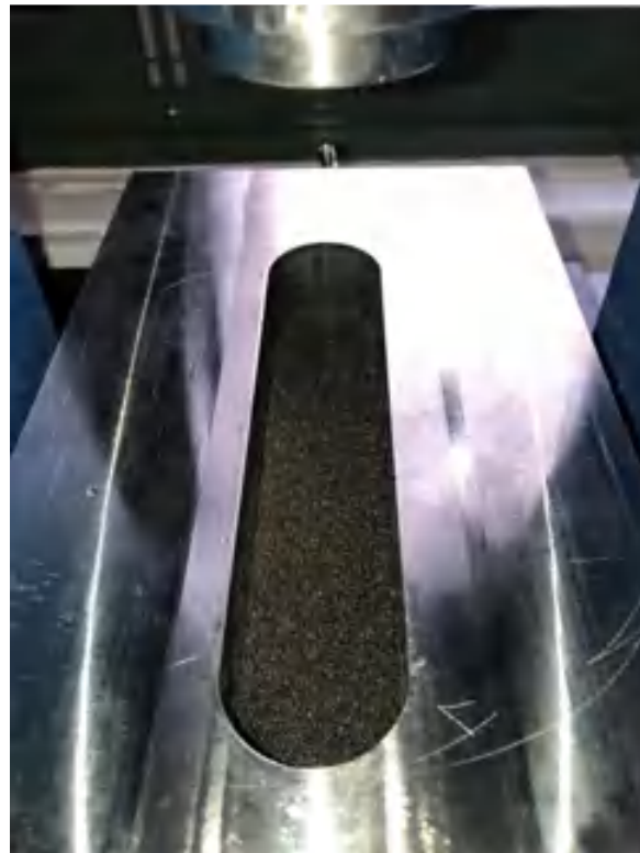
Fig. 73 Standard conductivity measurement cell (edited by the Author)
