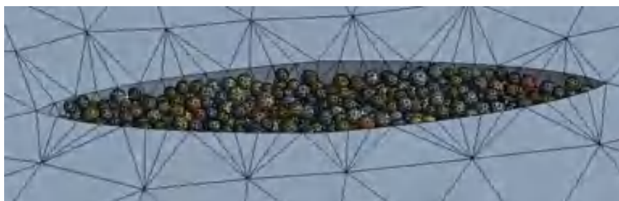
Fig. 60 Propped fracture in ANSYS SS with fine mesh (edited by the Author)
