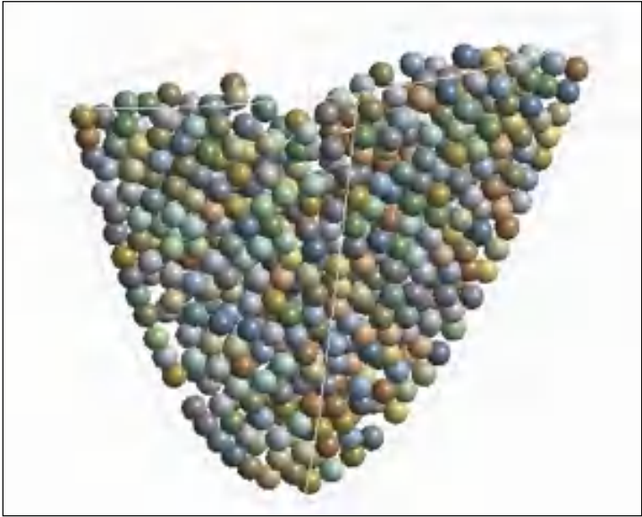
Fig. 35 Fracture filled by proppant (edited by the Author)
