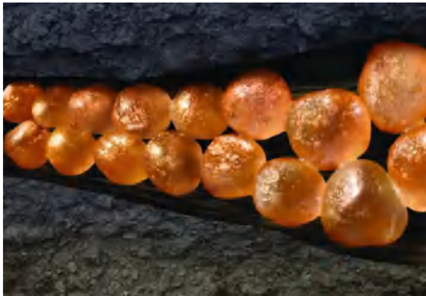
Fig. 2 Illustration of a propped fracture (Terracina & Harper, 2018)
