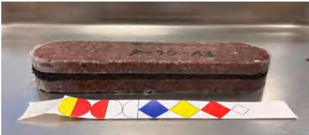
Fig. 72 Proppant between cores from the Kővágószőlős Formation (edited by the Author)
