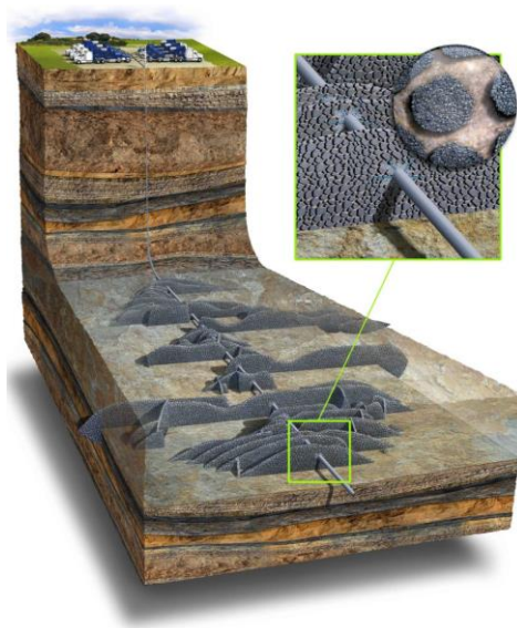
Fig. 1 Schematic of hydraulic fracturing (Schlumberger, 2021)
