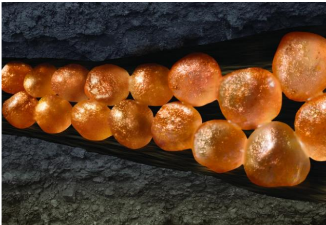
Fig. 2 Illustration of a propped fracture (Terracina & Harper, 2018)
