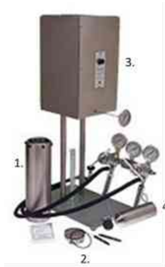
4. ábra: Permeability Plugging Test; (Model: 17-50-1)
