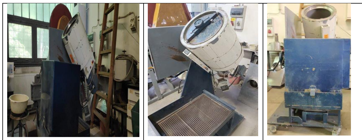
Figure 6.5. Tumbling laboratory ball mill
