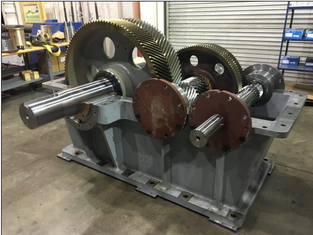
Figure 3 A typical double-reduction gearbox used in sucker-rod pumping (Pidenergy, 2016)
