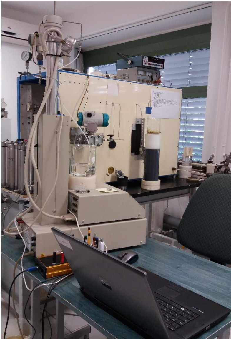
Fig. 20: Hassler Core holder Machine for measuring permeability
