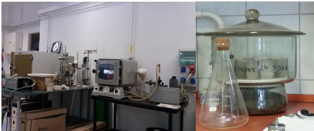
Fig. 18: Vacuum Machine to evacuate the core samples and dried out.
