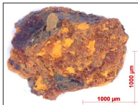
FIG.15: Strongly oxidized and Fe-oxide coated grain of BOL 1-8 (39X)
