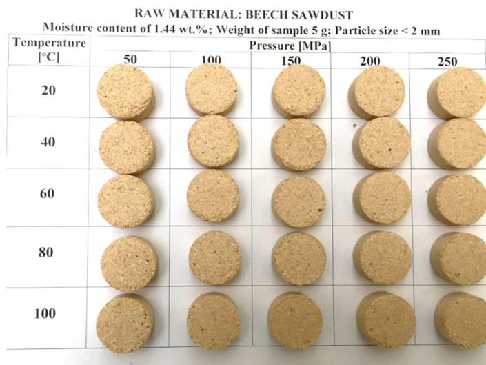
Figure 6.1. Tablets made from beech sawdust ( $x < 2$  mm)
