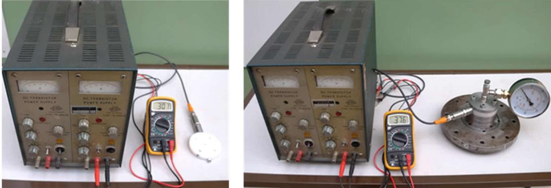
**Figure 4.11.** Set up pressure value in the backup pressure measurement disc (left) and hydraulic pressure calibration system (right)
