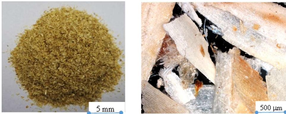
**Figure 3.1.** Spelt chaff with particle size  $< 1.6$  mm; (left) optical camera; (right) optical microscope: Zeiss AXIO Imager.M2m
