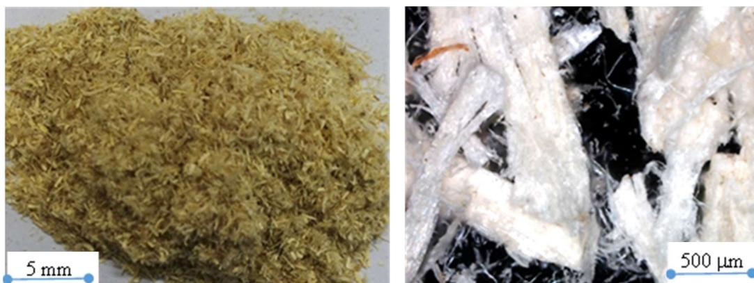
**Figure 3.6.** *A. mangium* sawdust ( $x < 1.6$  mm) in the case of one month seasoned wood; (left) optical camera; (right) optical microscope: Zeiss AXIO Imager.M2m
