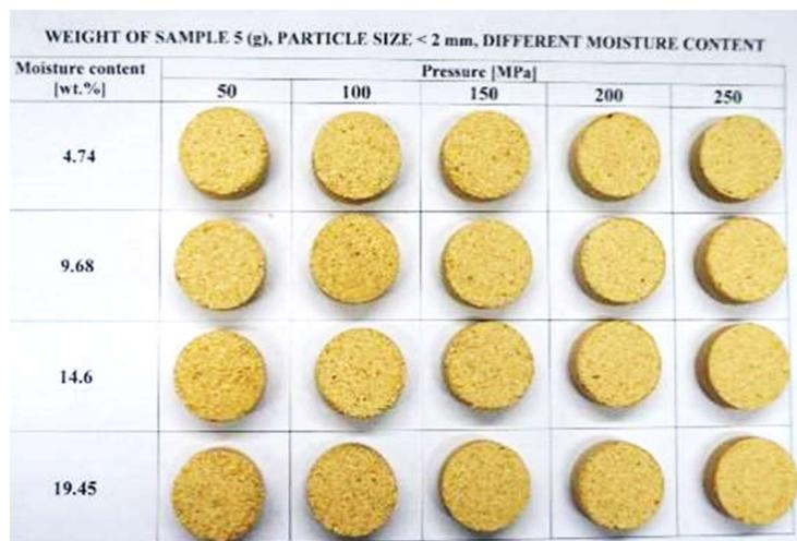
Figure 5.1. Tablets made from beech sawdust ( $x < 2$  mm)
