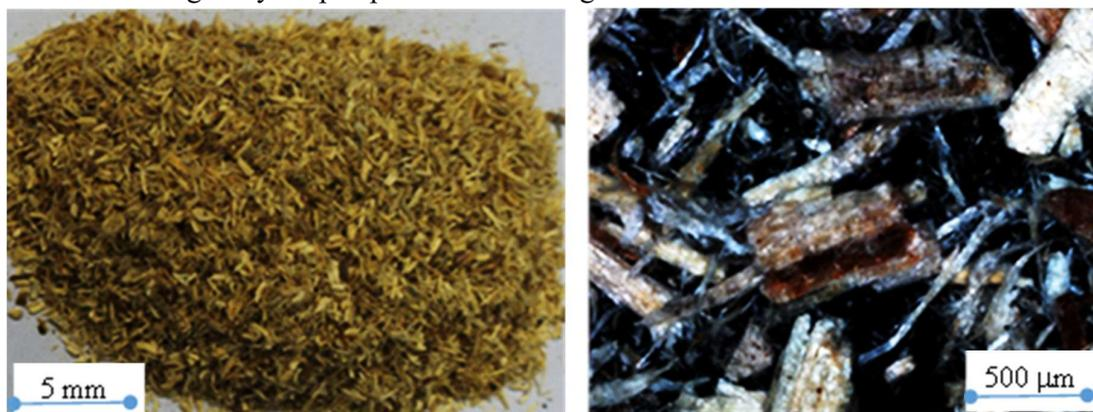
**Figure 3.7.** *A. mangium* sawdust with ( $x < 1.6$  mm) in the case of six months seasoned wood; (left) optical camera; (right) optical microscope: Zeiss AXIO Imager.M2m
