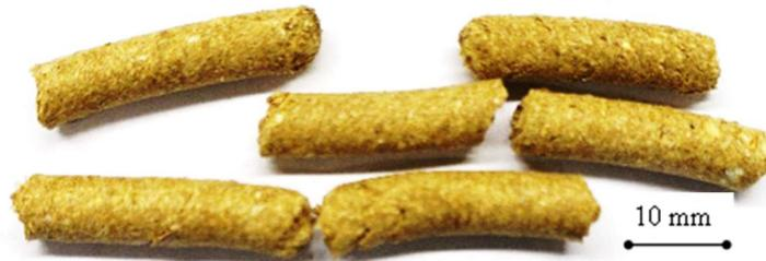
Figure 4.4. Pellets made from spelt chaff raw material by flat die pelletizer
