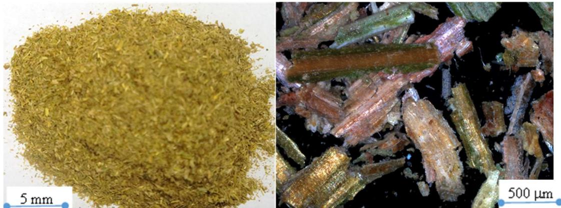
Figure 3.9. Rice straw with ( $x < 1.6$  mm); (left) optical camera; (right) optical microscope: Zeiss AXIO Imager.M2m
