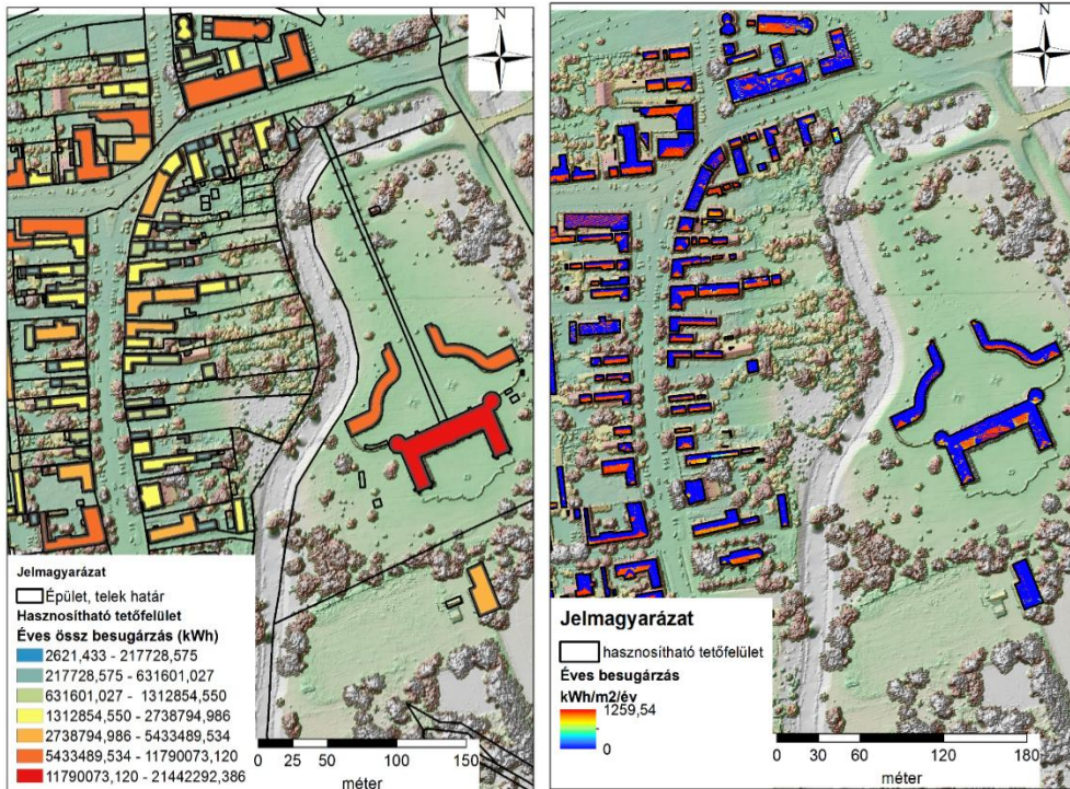
Figure 4: Showing yearly global radiation amount falling on roof surfaces (left) and global radiation amount falling on SE-SW exposed, flat and 35-43° roof surfaces (right), prepared by: Szalontai L.
