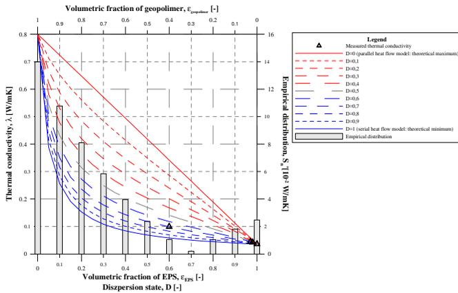
Figure 4.4.: Comparison of measured and theoretical resultant thermal conductivities in function of volumetric fraction of geopolimer and EPS in case of laboratory samples.
