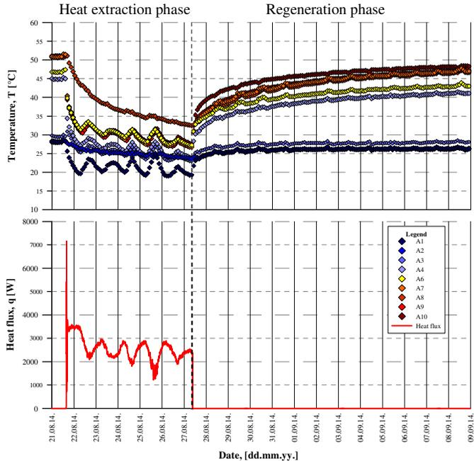
Figure 4.6.: Measured temperatures and extracted heat flux in heat well A as function of time.
