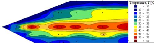
Figure 2.1.: Thermal profile of a typical MSW landfill (Yesiller et al., 2015b)
