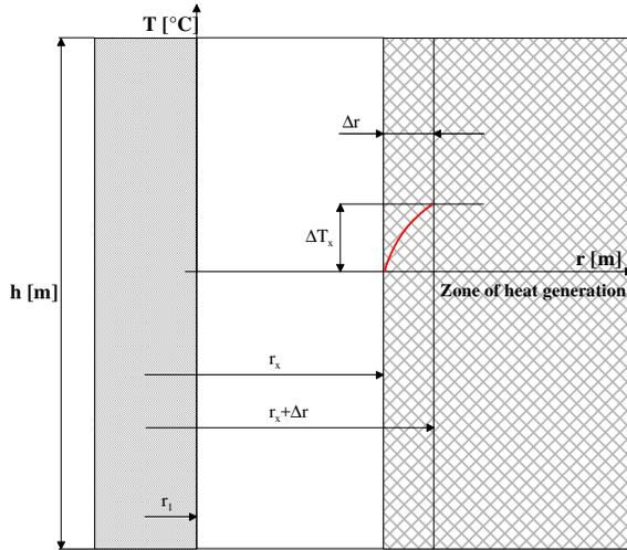
Figure 4.5.: The „tube shell with heat generation” model.
