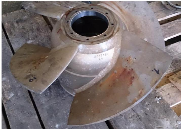
*Figure 1. The damaged turbine blades*
