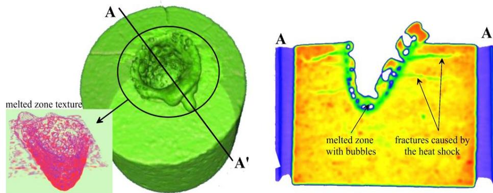
Figure 6. The 3D structure and the cross section of the laser treated sandstone sample on computed tomography images
