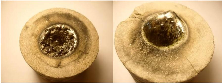
Figure 4. Laser drilled holes with melted smooth and bubble containing surfaces with and without heat shock induced fractures
