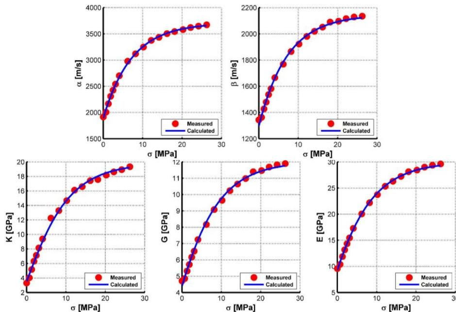
*Figure 3 Pressure dependent velocities and elastic moduli for the Berea sandstone*
