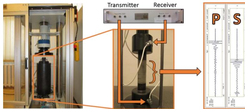
**Figure 1** Experimental setup. Left: load frame and pressure cell. Middle: ultrasonic device, sandstone sample between transmitter and receiver built in the pressure stamps. Right: P and S wave arrivals.
