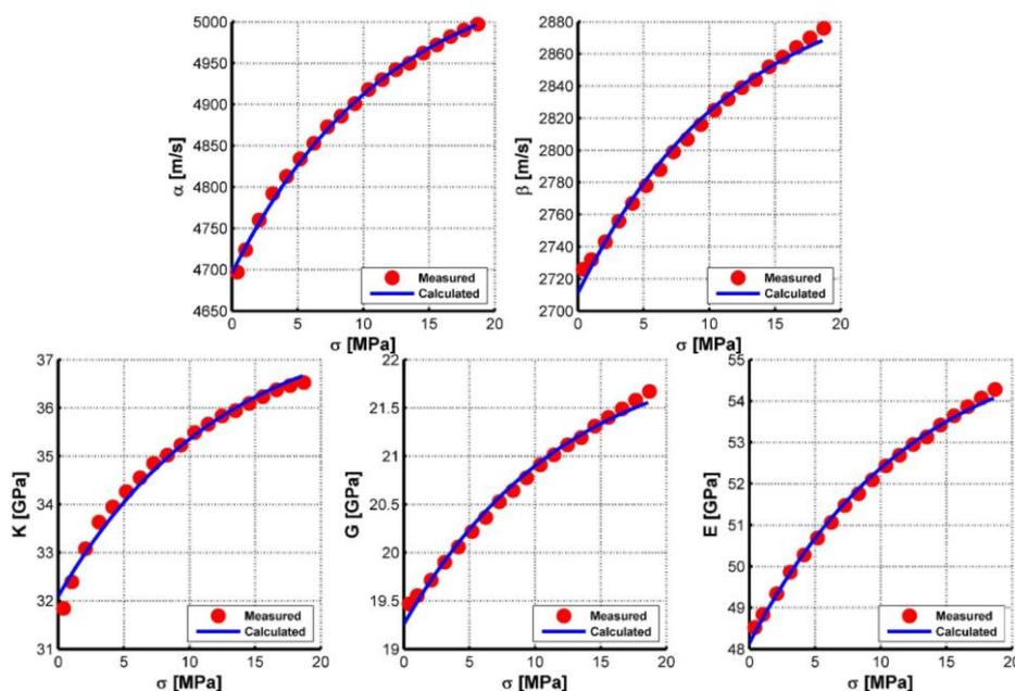
**Figure 2** Pressure dependent velocities and elastic moduli for sample A
