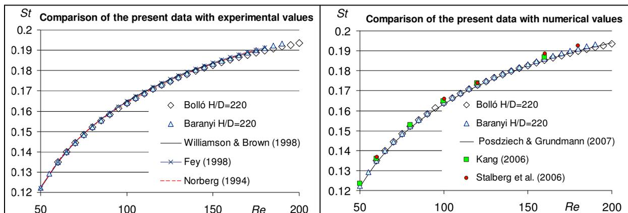
Fig. 2. Vortex shedding frequency versus Reynolds numbers
