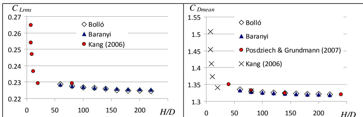
Fig. 3.  $C_{Lrms}$  and  $C_{Dmean}$  versus  $H/D$  at  $Re = 100$
