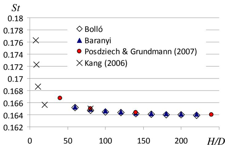
**Fig. 1.** Vortex shedding frequency versus  $H/D$  at  $Re = 100$
